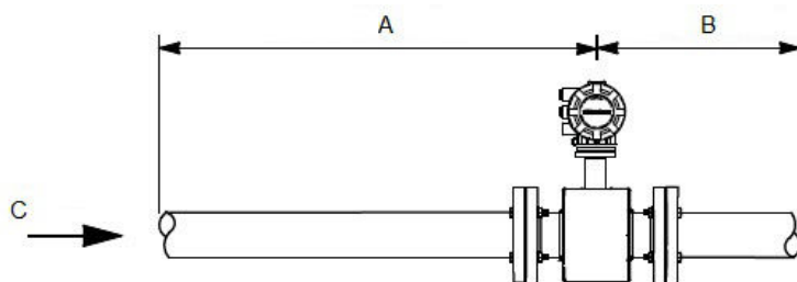
Figure 3-1: Upstream and Downstream Straight Pipe Diameters
